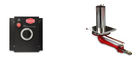
The AUTOMATIC (E series) burner works off 110V power. The desired temperature is set and the flame activated on an electronic display. A probe set into the dome instructs the valve to open or close, and the burner reaches and maintains the desired temperature. We call this "set and forget".
